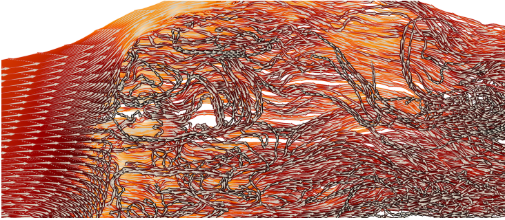
Figure 5.10: Streamlines depicted through light gray arrow shapes combined with a halo colored with a color map to depict velocity.
