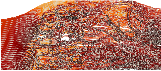
Figure 7: Streamlines depicted through light gray arrow shapes combined with a halo colored with a color map to depict velocity.
